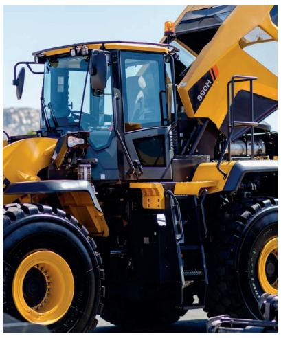
Access to the front of the cab by the operator or service person is a new feature. The same anti-slip bars used on the egress steps are used here for maximum anti-slip protection.
