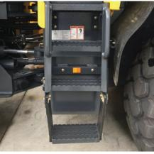
Access to the front of the cab by the operator or service person is a new feature. The same anti-slip bars used on the egress steps are used here for maximum anti-slip protection.
