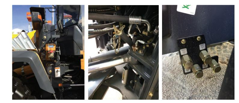
All pressure taps and sight gauges are easily accessible. Fluid drains provide environmentally friendly drainage capability and are grouped together for convenient serviceability.
